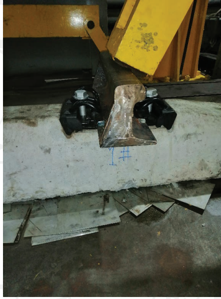
Railway sleeper and component durability test (including rails, elastic pads, bullet bars and fastening screws)
