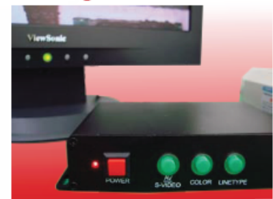
X-Y cross-line generator
